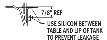
Sectional View Showing Table Connections
